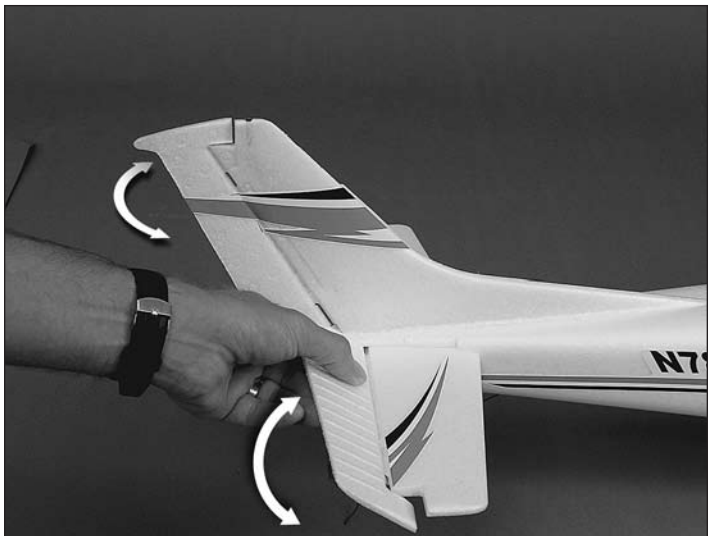
❑ 6. Move the rudder back-and-forth and the elevator up-and-down to make certain everything is operating smoothly. If there is much resistance or if something doesn't seem right, remove the fin and stab from the fuselage and make sure you have the pushrods hooked up correctly. Then reinstall and try again.
