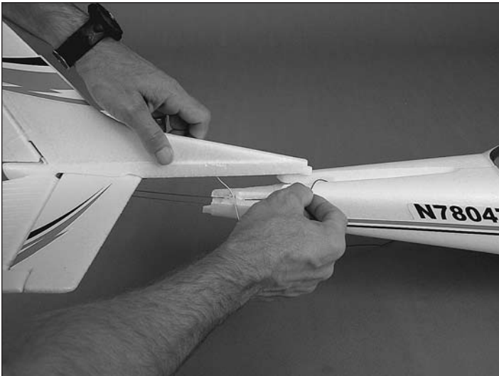
❑ 4. Just before the fin and stab are all the way into position, reach inside the fuselage with small needle-nose pliers or hemostats and feed the pushrods into the pushrod connectors already mounted on the servos.
